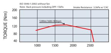
**ENGINE SPEED (rpm)**
